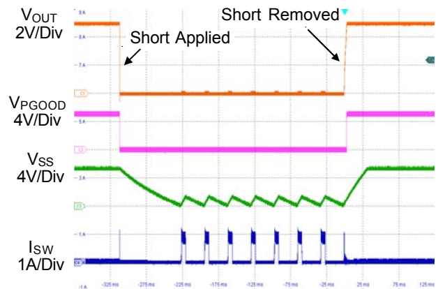
Figure 3. Short-Circuit Protection and Recovery
