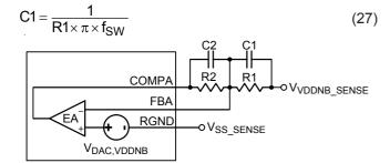
Figure 19. VDDNB Controller: Compensation Circuit
