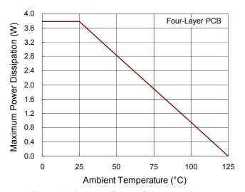
Figure 24. Derating Curve of Maximum Power Dissipation
