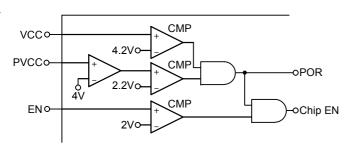
Figure 1. Power Ready (POR) Detection
