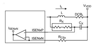
Figure 14. VDD Controller: Lossless Inductor Sensing
