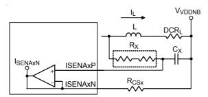
Figure 21. VDDNB Controller: Lossless Inductor Sensing
