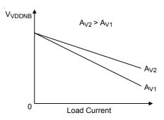
Figure 18. VDDNB Controller: Error Amplifier gain (A<sub>V</sub>) Influence on V<sub>VDDNB</sub> Accuracy
