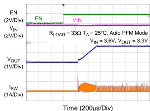
Start-Up Waveforms (Heavy Load)
