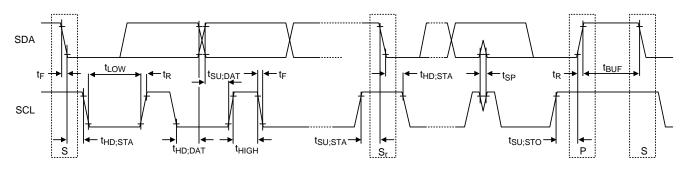
Figure 6. I<sup>2</sup>C Read and Write Stream and Timing Diagram
