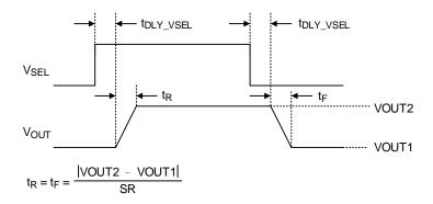
Figure 5. DVS Control the VSEL Pin
