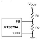
Figure 1. Setting the Output Voltage
