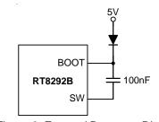
Figure 2. External Bootstrap Diode
