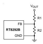
Figure 1. Output Voltage Setting
