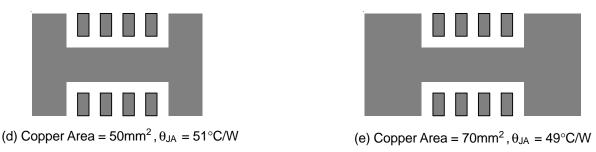
Figure 6. Themal Resistance vs. Copper Area Layout Design
