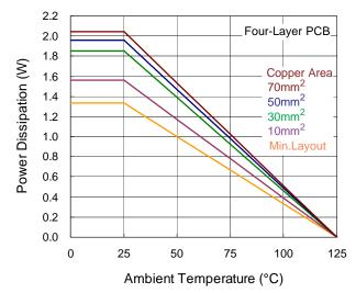
Figure 7. Derating Curves for RT8292B Package
