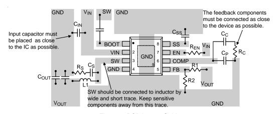
Figure 8. PCB Layout Guide
