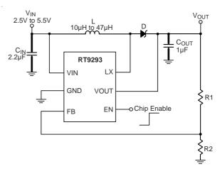
Figure 5. Constant Output Voltage Application
