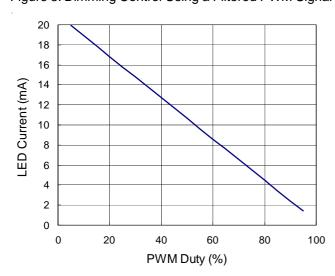
Figure 4. PWM Duty Cycle vs. LED Current
