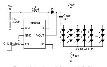
Figure 6. Application for Driving 3 X 13 WLEDs
