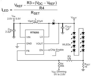
Figure 2. Dimming Control Using a DC Voltage
