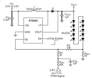
Figure 3. Dimming Control Using a Filtered PWM Signal
