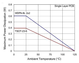
Figure 7. Derating Curves for RT9293 Packages
