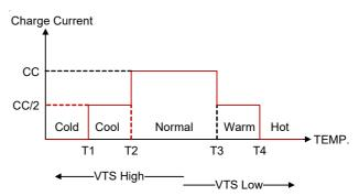
Thermal of battery can be monitored by TS PIN. There are 4 sections should be implemented in JEITA function. Base on  $R_{hot}$  and  $R_{cold}$ , RT1 and RT2 can be determined by equation (1) and equation (2).
