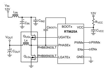
Figure 6. Synchronous Buck Converter Circuit
