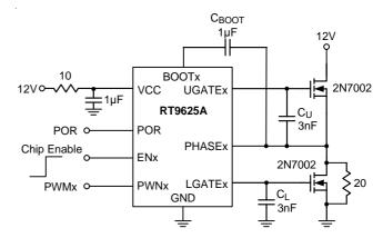
Figure 3. Power Dissipation Test Circuit
