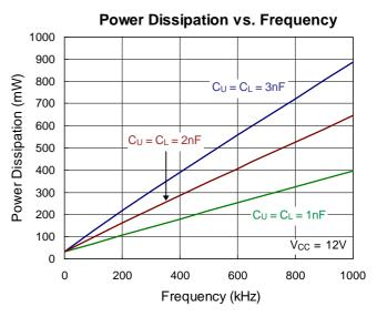
Figure 4. Power Dissipation vs. Frequency
