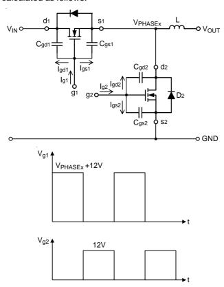
Figure 1. Equivalent Circuit and Waveforms (V<sub>CC</sub> = 12V)
