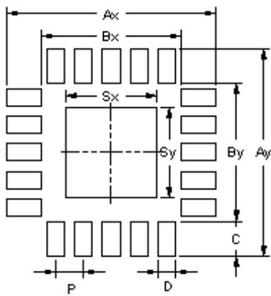
**V/W/X QFN-4x4-24L / V/W QFN-5x5-24L**
