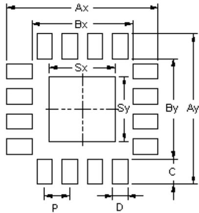
**V/W/X QFN-3x3-20L / V/W QFN-4x4-20L**
