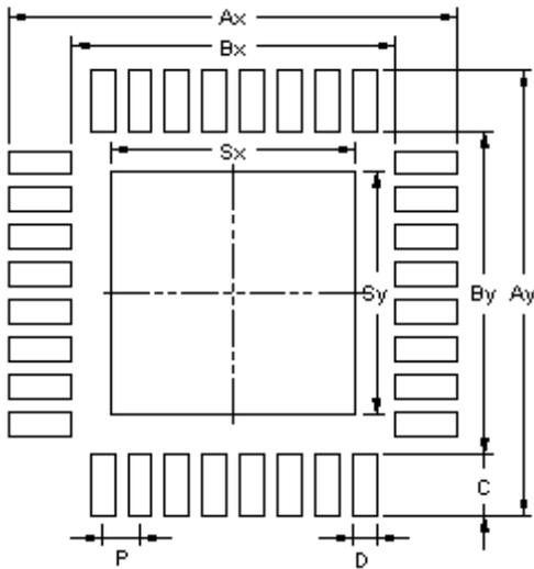
**V/W QFN-5x5-40L / V/W QFN-6x6-40L**
