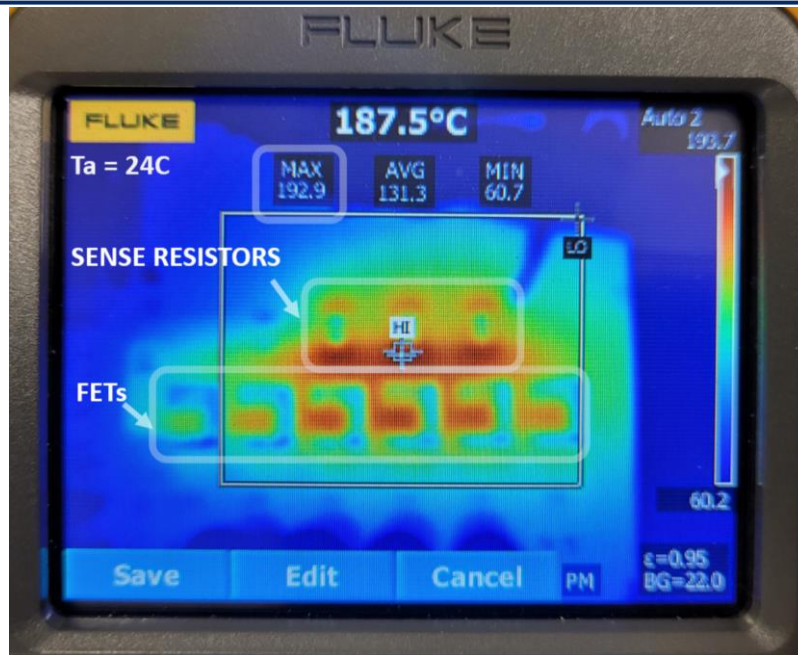
Figure 14. Example of a Soft Short and Potential Failure with Other Hot Swap Controllers Having Only One Level of Overcurrent Protection ( I_{LIM}=300A ). MOSFET Case Temperature Reaching 180°C, at 285A after 4 Minutes.
