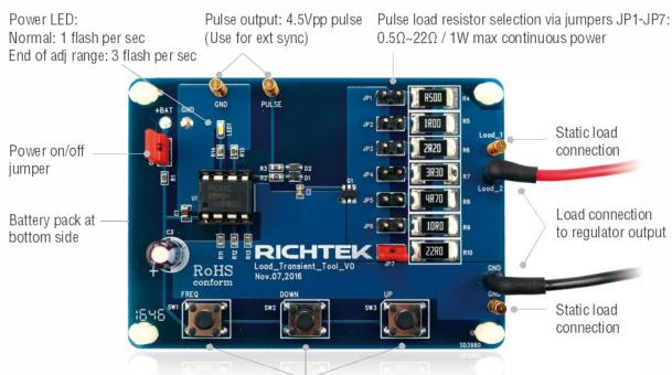
Press UP or DOWN button: Duty-cycle adjust 0.1% ~ 50% Press FREQ + UP or DOWN button: Frequency adjust 15Hz / 61Hz / 244Hz / 976Hz
