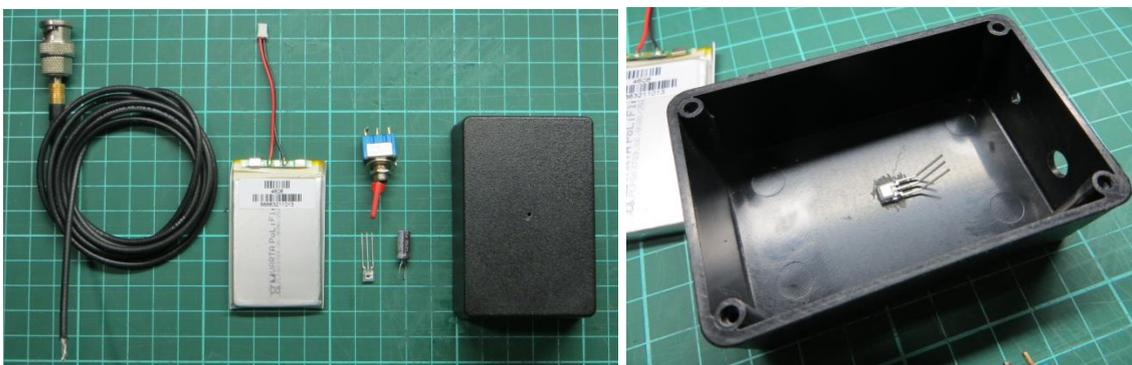
Required components: coaxial wire, Li-ION battery, TSL257 IC, a switch, a 22uF/25V electrolytic capacitor and a black plastic box with a 3mm hole drilled in the top. The TSL257 is placed with the sensor towards the hole.
