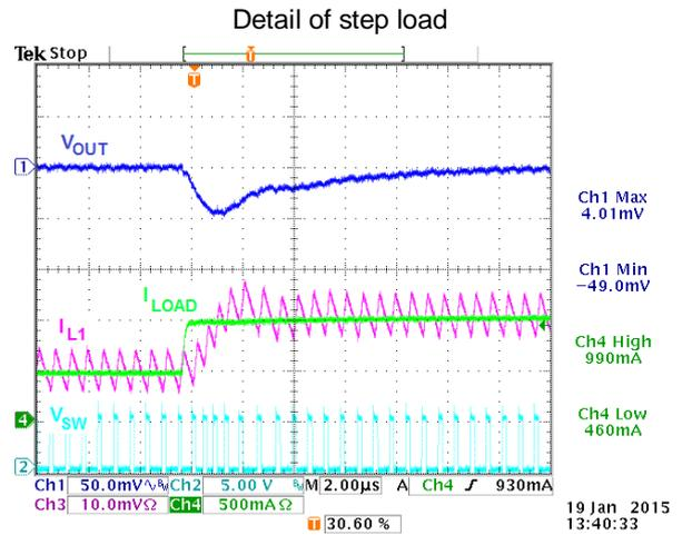
Frequency will increase during transient, thereby increasing duty-cycle.
