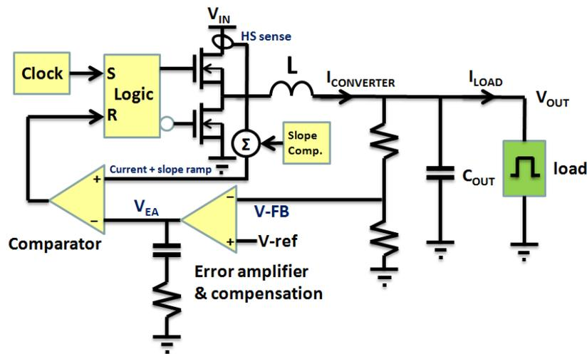
Figure 1. Current Mode Block Diagram
