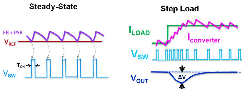
Figure 6. ACOT Steady-State and Load Transient Waveforms
