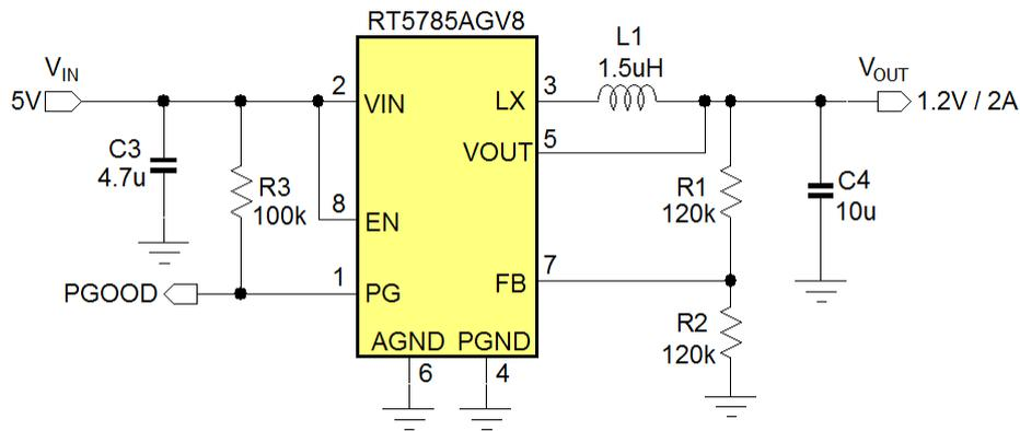
Figure 11: RT5785A 5V→1.2V/1A Application
