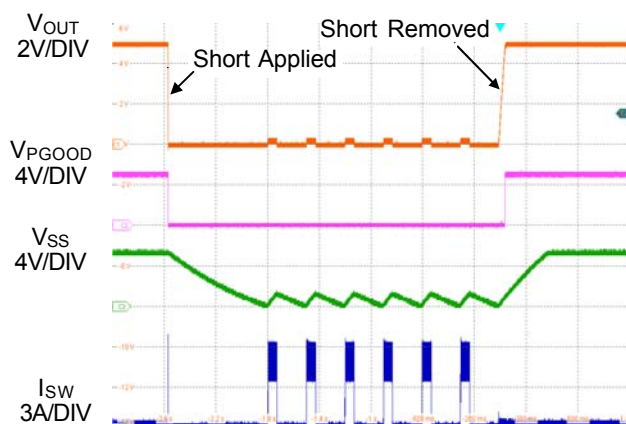
Figure 3. Short-Circuit Protection and Recovery
