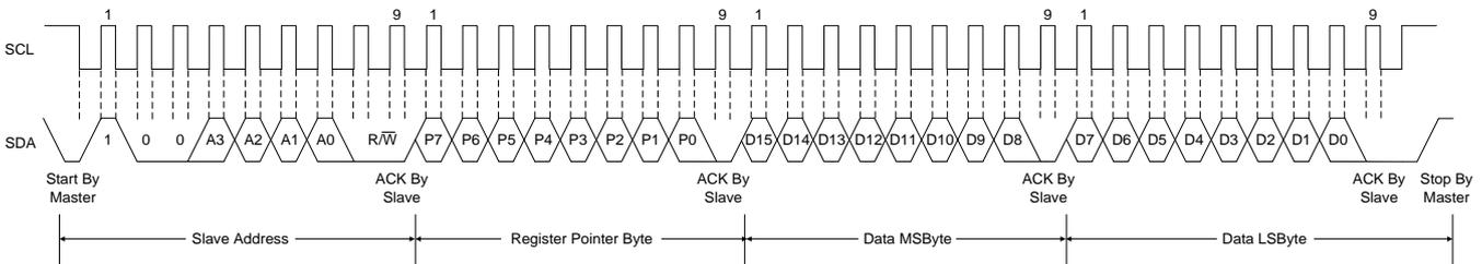
Figure 4. Timing Diagram for Write Word Format
