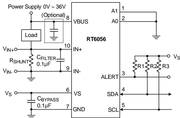
Note : All the input and output capacitors are the suggested values, referring to the effective capacitances, subject to any de-rating effect, like a DC Bias.
