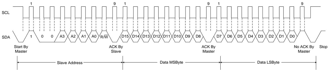
Figure 5. Timing Diagram for Read Word Format
