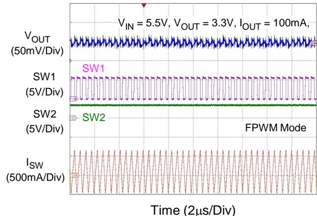
**PWM Switching Waveforms
