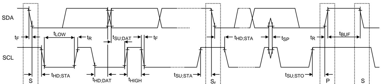
Figure 6. I<sup>2</sup>C Read and Write Stream and Timing Diagram
