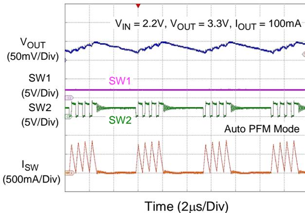
**PWM Switching Waveforms
