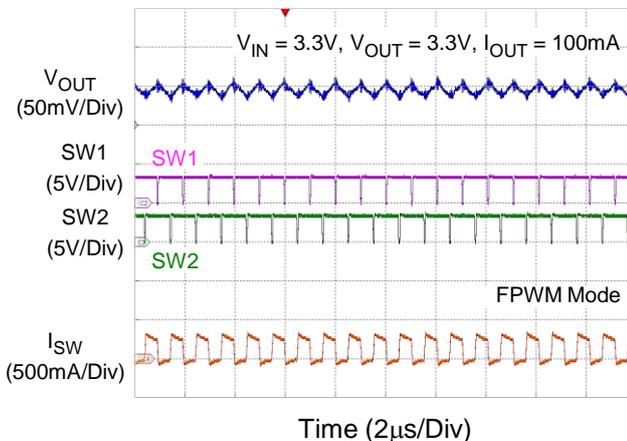
**PWM Switching Waveforms
