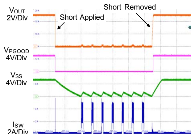
Figure 3. Short Circuit Protection and Recovery
