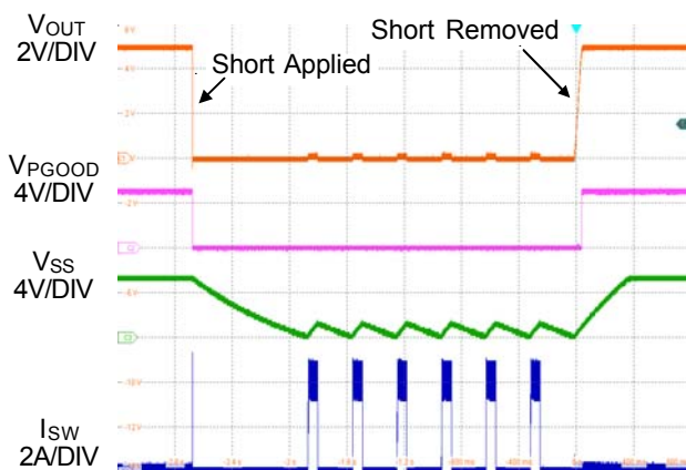
Figure 3. Short Circuit Protection and Recovery
