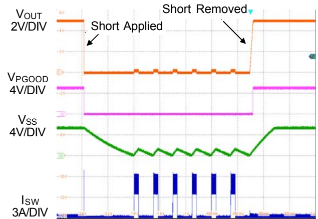
Figure 3. Short-Circuit Protection and Recovery
