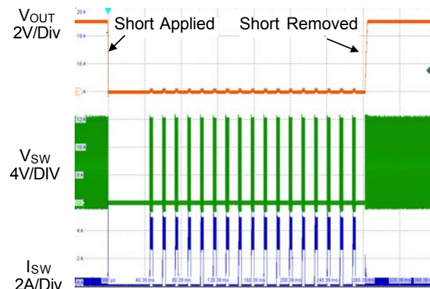
Figure 2. Short-Circuit Protection and Recovery
