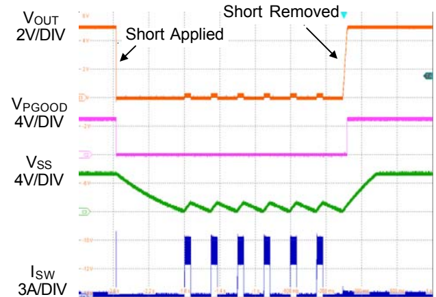
Figure 3. Short-Circuit Protection and Recovery
