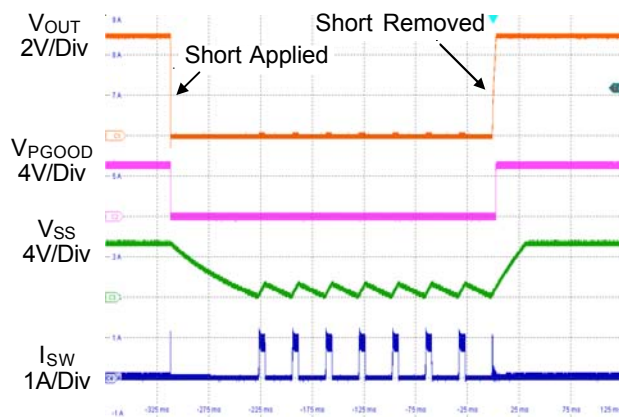
Figure 3. Short Circuit Protection and Recovery
