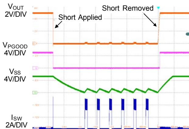
Figure 3. Short-Circuit Protection and Recovery
