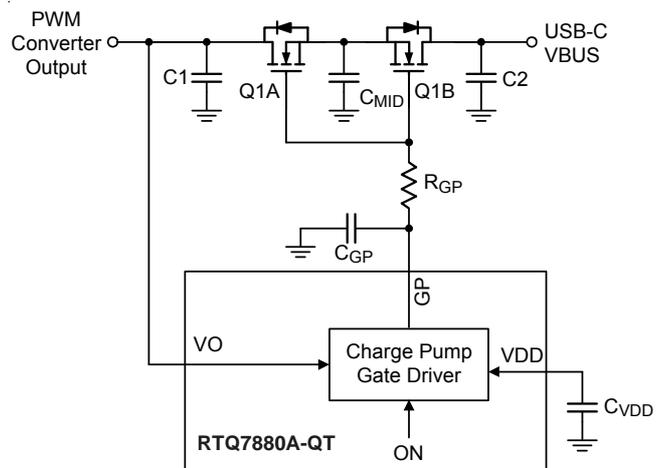
Figure 4. Functional diagram of the power-path control
