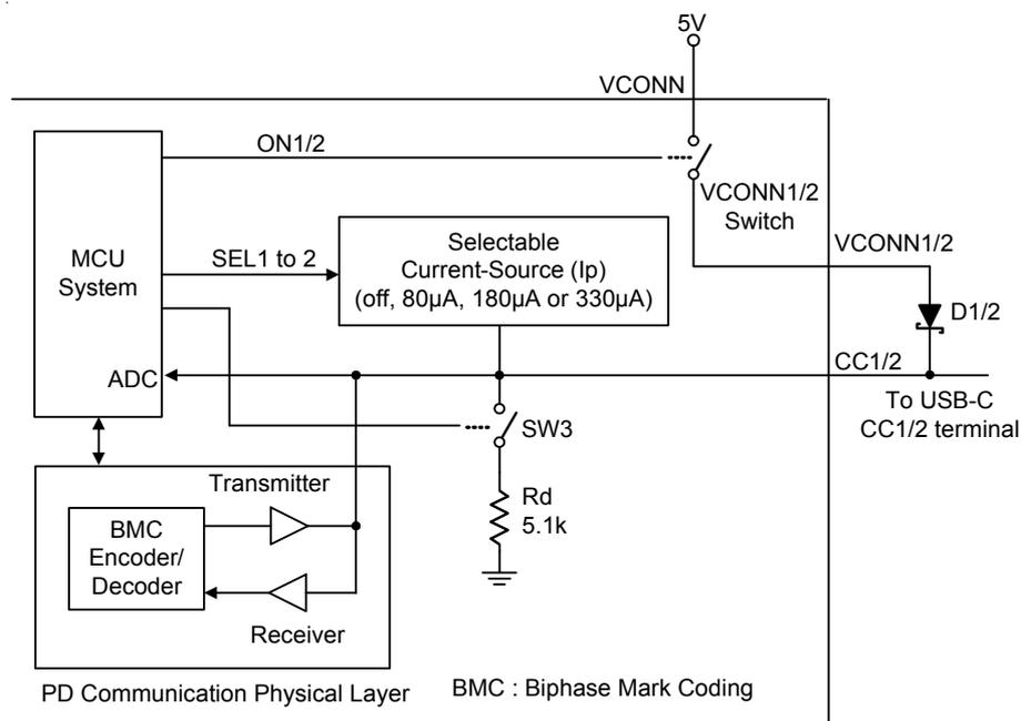
Figure 2. Functional diagram of VCONN and CC1/2 functions
