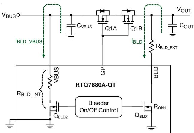
Figure 3. Functional diagram of the output bleeders
