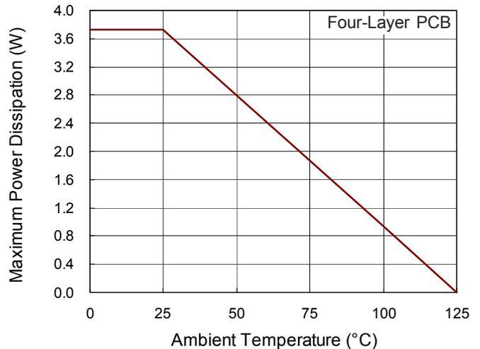
Figure 5. Derating Curve of Maximum Power Dissipation
