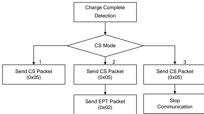
Figure 15. Operation Modes of Charge Complete Detection
