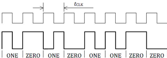
Figure 11. Example of the Differential Bi-phase Encoding
