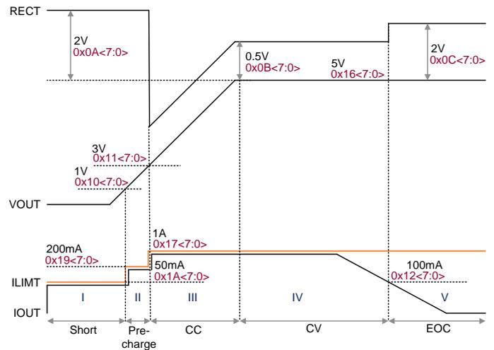
Figure 13. Battery Charge Behavior
