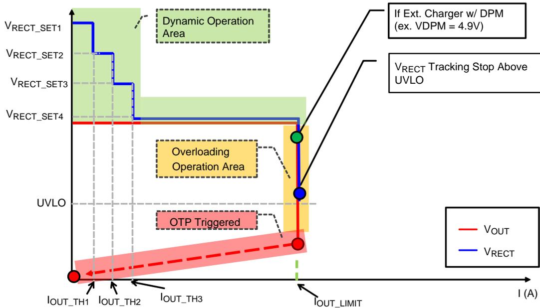
Figure 4. Dynamic Rectifier Voltage vs. Output Current
