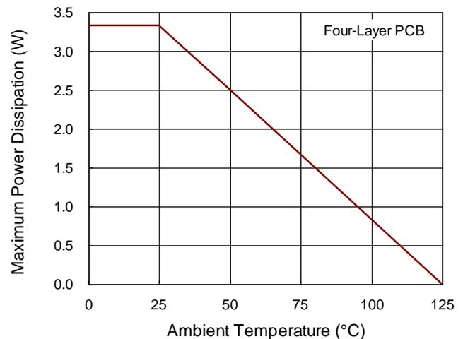
Figure 16. Derating Curve of Maximum Power Dissipation
