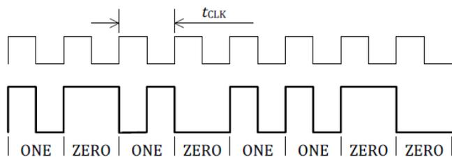
Figure 12. Example of the Differential Bi-phase Encoding
