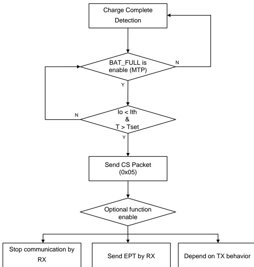
Figure 15. Operation Modes of Charge Complete Detection
