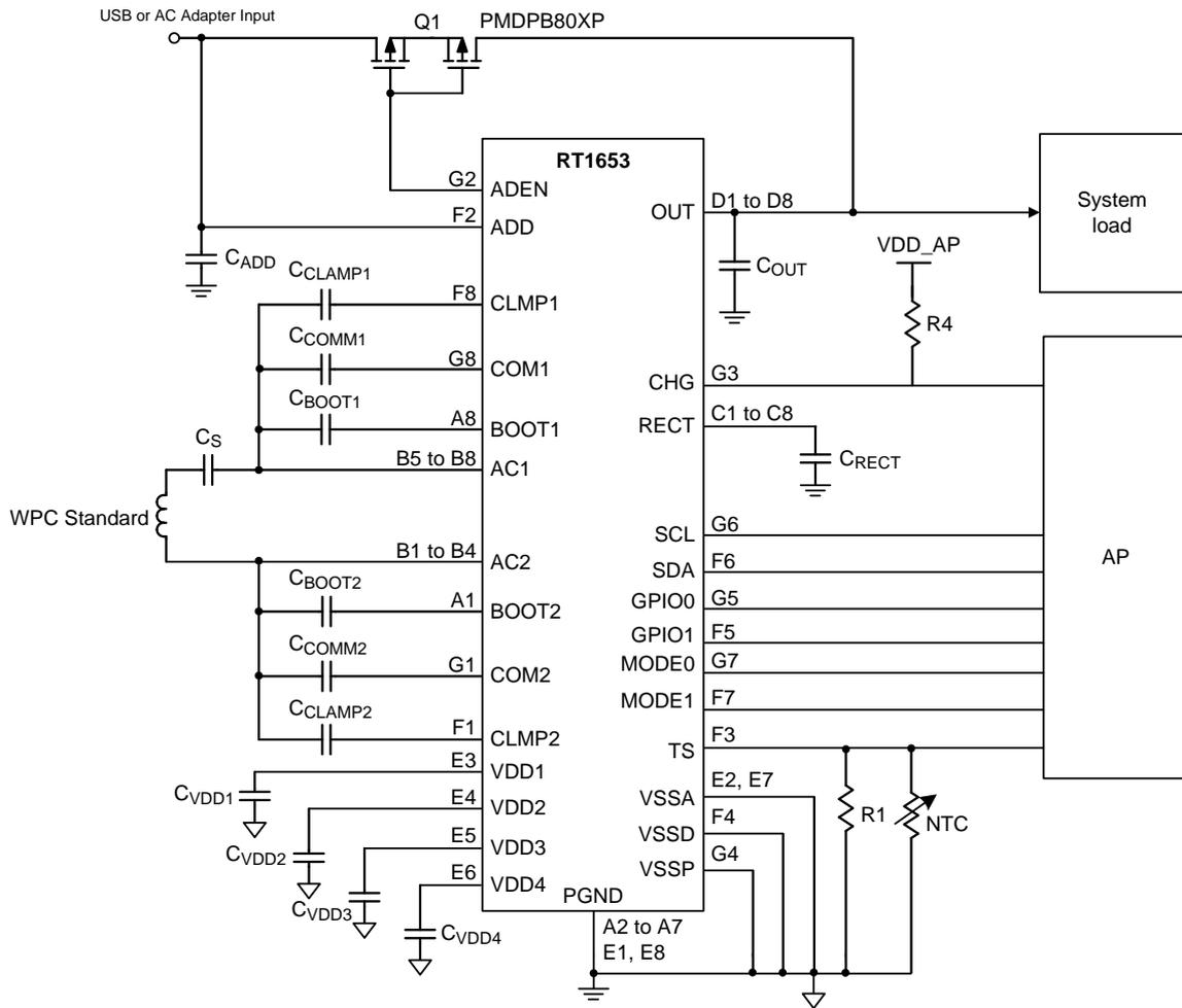
Note : The component value and the maximum voltage rating is based on the WPC standard transmitter and 5V adapter application. The customer should modify it depends on the different design and application.
