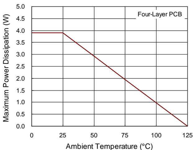
Figure 16. Derating Curve of Maximum Power Dissipation
