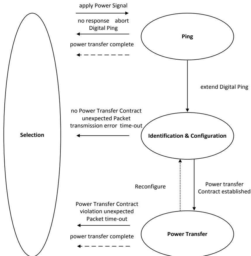
Figure 2. WPC V1.2.4 Low Power Transfer Phases
