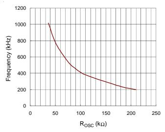
Figure 7. Switching Frequency vs. ROSC Resistor
