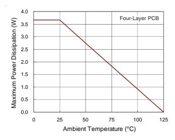
Figure 10. Derating Curve of Maximum Power Dissipation
