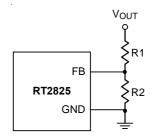
Figure 1. Setting the Output Voltage
