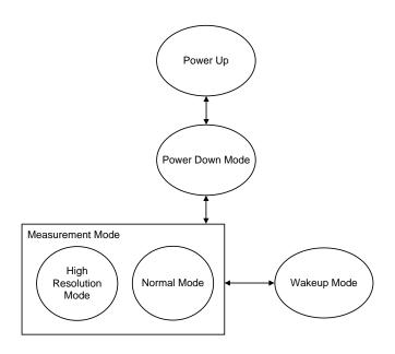
Figure 1 Operating Mode State Diagram
