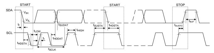
Figure 3. Timing Chart of the I<sup>2</sup>C
