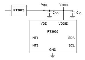
Figure 2. Single Power Supply Design Using the RT9078
