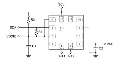
Note : The recommended value for C1 and C2 is  $0.1 \mu F$ .
