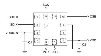
Note : The recommended value for C1 and C2 is  $0.1 \mu F$ .
