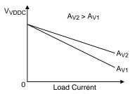
Figure 8. VDDC Controller: Error Amplifier gain (A<sub>V</sub>)
