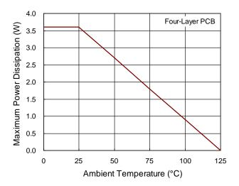
Figure 12. Derating Curve of Maximum Power
