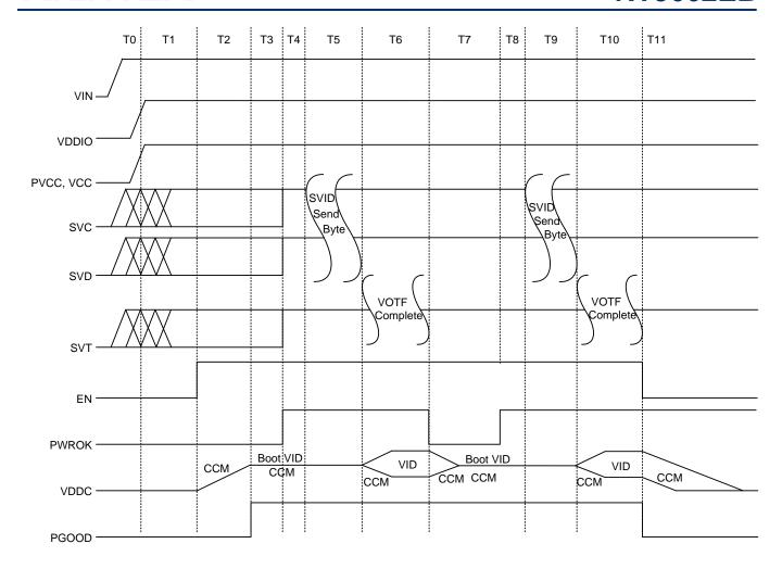
Figure 2. Simplified Sequence Timing Diagram
