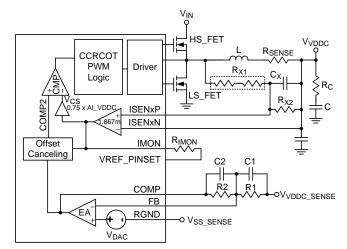
Figure 7.VDDC Controller : Simplified Schematic with Voltage Loop and Current Loop
