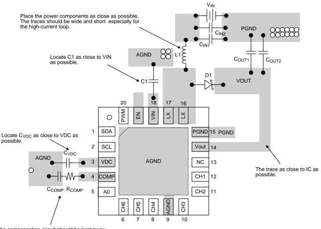
The compensation circuit should be kept away from the power loops and should be shielded with
