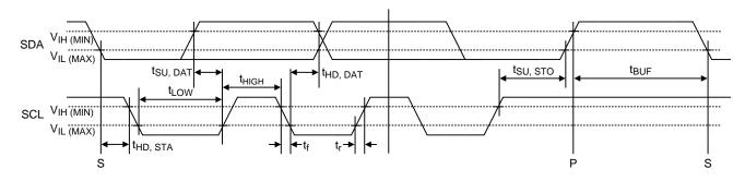
RT4527A I<sup>2</sup>C slave address = 7'b0110\_110(A<sub>0</sub> = 0) and 7'b0110\_111(A<sub>0</sub> = 1). I<sup>2</sup>C interface support fast mode (bit rate up to 400kb/s). The write or read bit stream (N  $\ge$  1) is shown below
