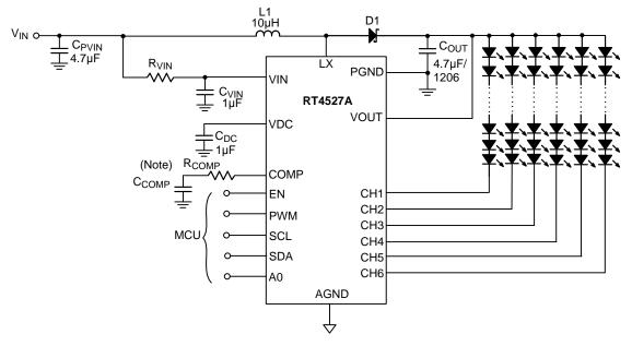
Note : RT4527A recommend to use differential compensation parameters for Low VIN application, For typical application, LED=6P11S, Boost Switching frequency = 1.225MHz, I<sub>LED</sub> =2 4mA/CH, C<sub>OUT</sub> = 4.7µF, L1 = 10µH, while the recommended value for compensation is as follows table:
