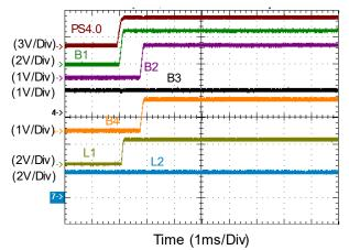
PS4.0 Power Off Sequence for GPIO3 = H
