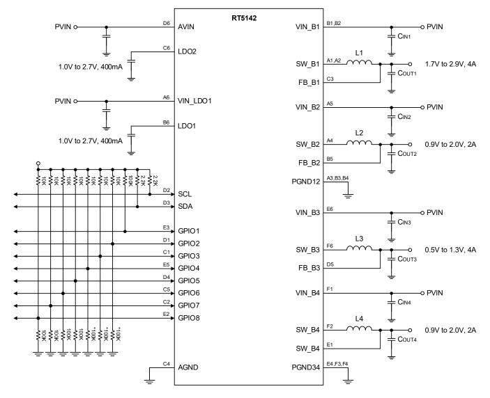
Note: \*: If GPIOx is set to High-Z, 100k should be removed.
