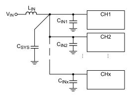
Figure 3. The Location of Input Bulk Capacitors Diagram
