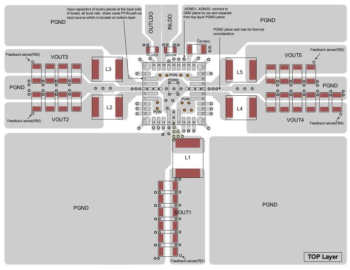
Figure 14. PCB Layout Reference of Option 1 (Top Layer)
