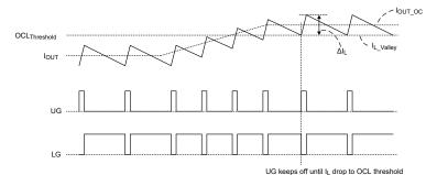
Figure 1. Cycle-by-Cycle "Valley" Current Limiting Control
