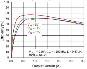
Buck5 Efficiency vs. Output Current in FCCM
