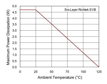
Figure 13. Derating Curve of Maximum Power Dissipation
