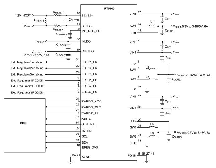
Figure 6. Application Circuit for Buck Dual-Phase Mode Operation
