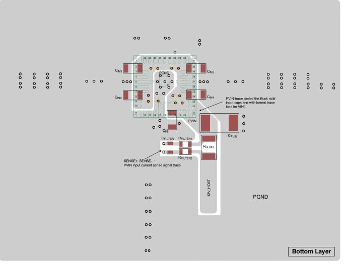
Figure 15. PCB Layout Reference of Option 1 (Bottom Layer, top view)
