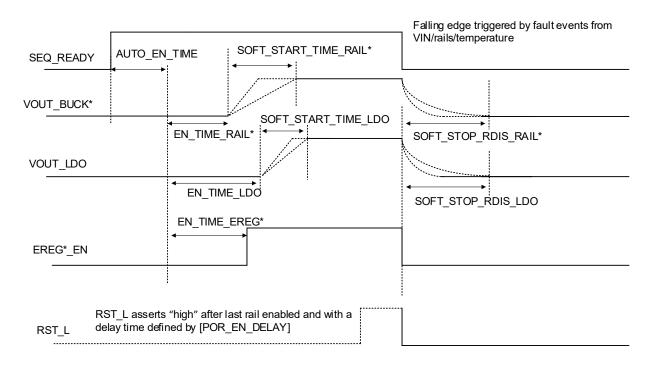
Figure 7. Rail Power-On and Power-Off Procedure
