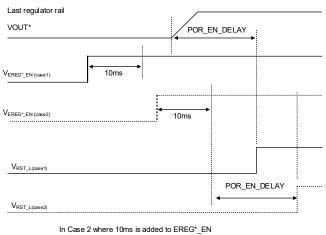
assertion, the external regulator requires start-up timing that is later than the PMIC's last regulator rail
