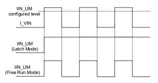
Figure 9. IIN\_LIM "Latch Mode" and "Free Run Mode" Operation
