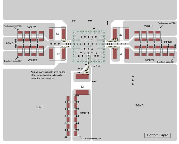
Figure 18. PCB Layout Reference of Option 2 (Bottom Layer, top view)
