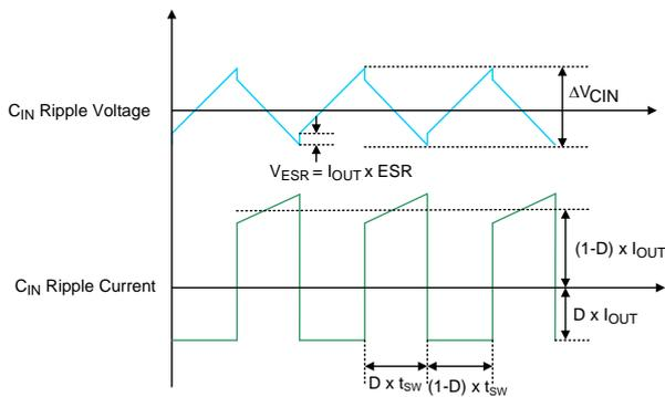
Figure 5. C<sub>IN</sub> Ripple Voltage and Ripple Current
