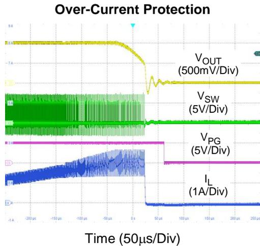
Figure 3. Over-Current Protection
