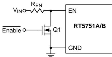
Figure 8. Logic Control for the EN Pin
