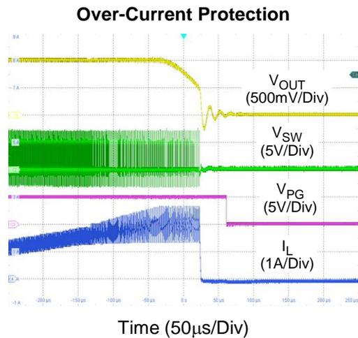
Figure 3. Over-Current Protection
