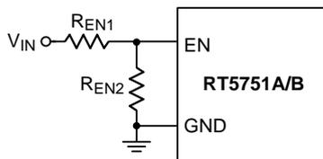
Figure 9. Resistive Divider for Under-Voltage Lockout Threshold Setting
