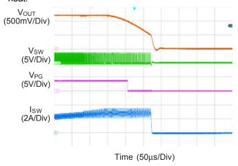
Figure 2. Over-Current Protection
