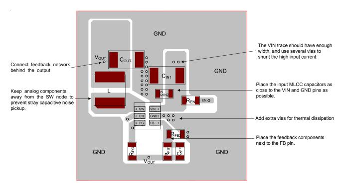
Figure 13. Layout Guide for UDFN-6L 1.4x1 (FC)
