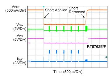
Figure 3. Short-Circuit Protection and Recovery
