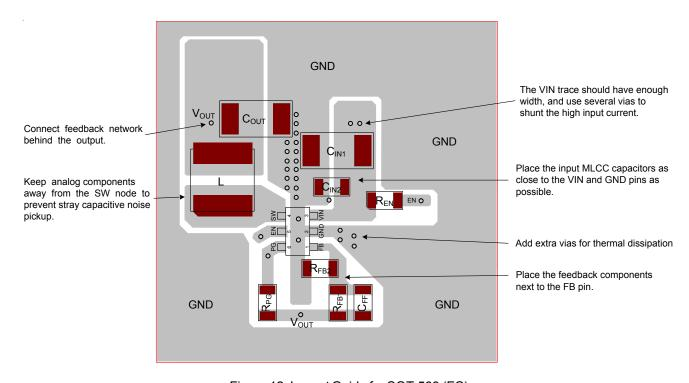
Figure 12. Layout Guide for SOT-563 (FC)
