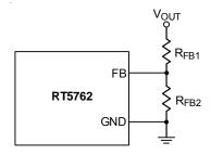
Figure 5. Output Voltage Setting
