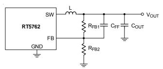
Figure 9. Feedback Loop with Feedforward Capacitor
