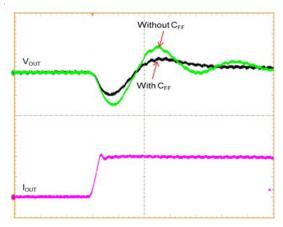
Figure 11. Load Transient Response with and without Feedforward Capactior
