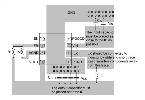
Figure 10. UDFN-8L 2.5x2 (FC) PCB Layout Guide
