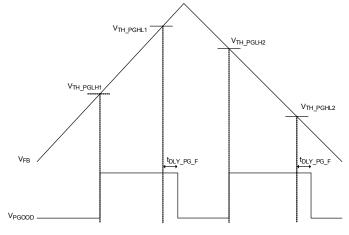
Figure 4. The Logic of PGOOD
