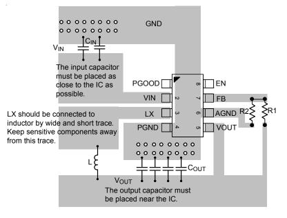
Figure 10. TSOT-23-8 (FC) PCB Layout Guide
