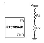
Figure 8. Output Voltage Setting
