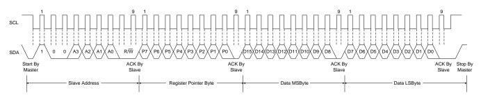
Figure 4. Timing Diagram for Write Word Format
