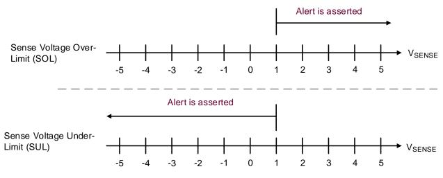
Figure 2. Alert Pin Response to SOL and SUL When the Alert Limit Register (07h) is Set to 1
