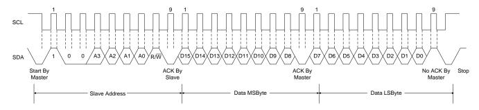
Figure 5. Timing Diagram for Read Word Format
