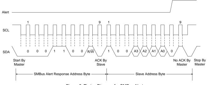
Figure 6. Timing Diagram for SMBus Alert
