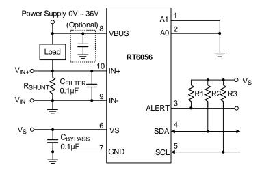
Note : All the input and output capacitors are the suggested values, referring to the effective capacitances, subject to any de-rating effect, like a DC Bias.
