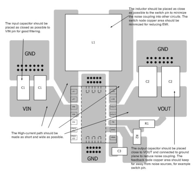
Figure 2. PCB Layout Guide
