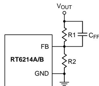
Figure 1. C<sub>FF</sub> Capacitor Setting
