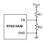
Figure 5. Output Voltage Setting
