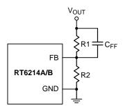
Figure 1. CFF Capacitor Setting
