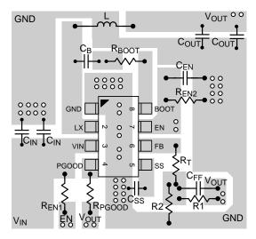
Figure 10. PCB Layout Guide for TSOT-23-8 package
