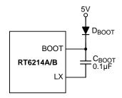
Figure 6. External Bootstrap Diode
