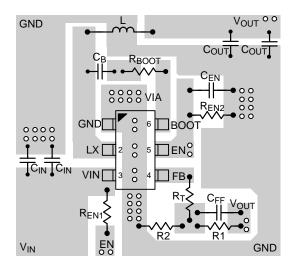
Figure 9. PCB Layout Guide for TSOT-23-6 package
