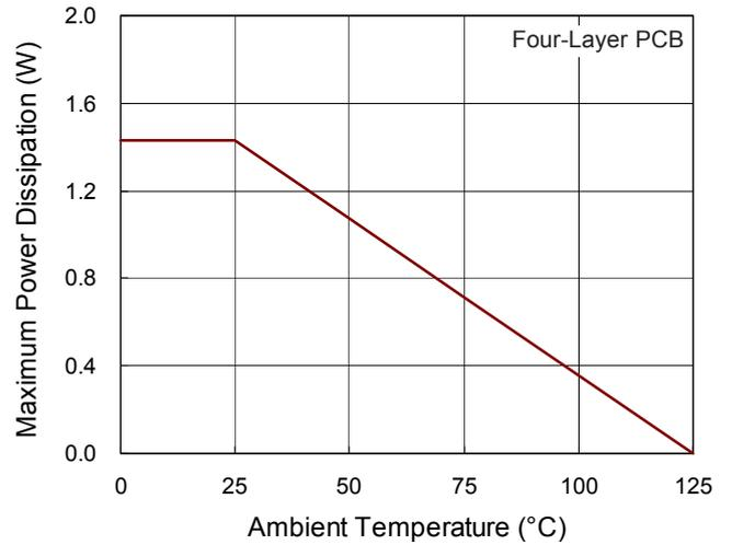
Figure 7. Derating Curve of Maximum Power Dissipation
