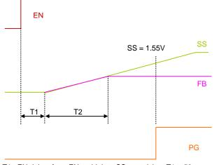
T1 : EN delay, from EN go high to SS start rising, T1 = 50 $\mu$ s; T2 : normal SS, from FB rising to settled, T2 = C<sub>SS</sub> x 0.9/I<sub>SS</sub>; PG go high after SSOK (SS = 1.55V)
