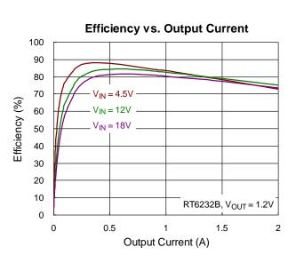
Efficiency vs. Output Current
