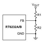
Figure 5. Output Voltage Setting
