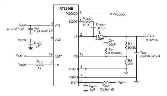
Note : All the input and output capacitors are the suggested values, referring to the effective capacitances, subject to any derating effect, like a DC bias.
