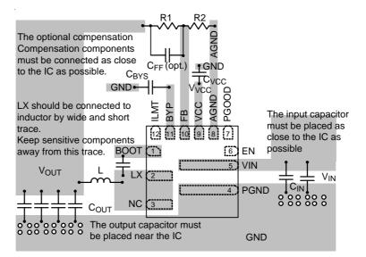
Figure 3. PCB Layout Guide
