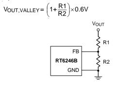
Figure 1. Output Voltage Setting
