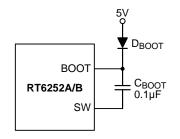
Figure 10. External Bootstrap Diode
