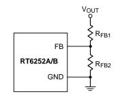
Figure 2. Output Voltage Setting
