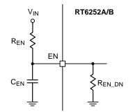
Figure 7. External Timing Control
