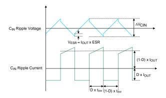
Figure 1. CIN Ripple Voltage and Ripple Current
