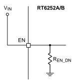
Figure 6. Automatic Start-Up Setting
