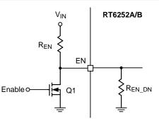
Figure 8. Digital Enable Control Circuit
