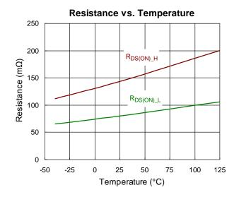
Figure 13. RT6252A/B RDS(ON) vs. Temperature
