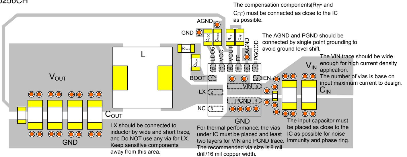
Figure 9. Layout Guide of RT6256CH
