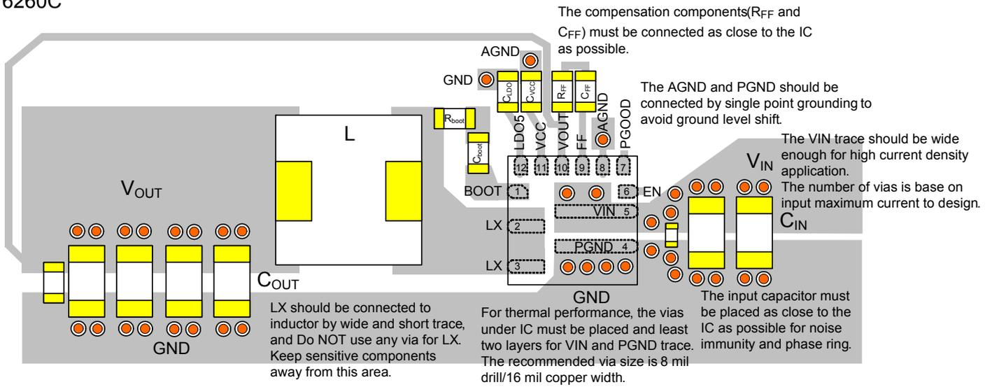
Figure 8. Layout Guide of RT6260C
