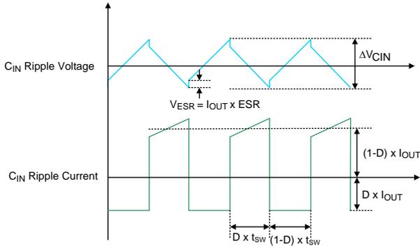
Figure 1. C<sub>IN</sub> Ripple Voltage and Ripple Current
