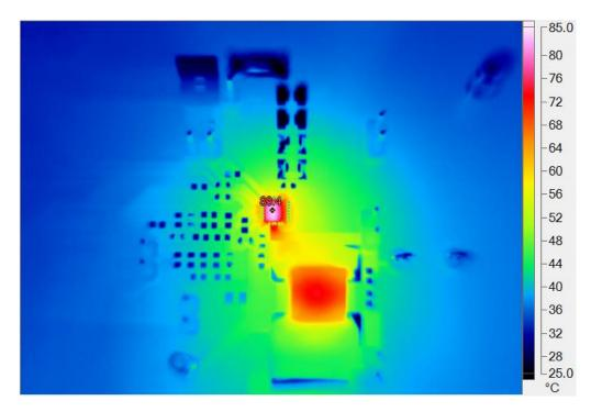
Figure 25. Thermal image of RT6310B/BH with VOUT = 3.3V, VIN = 19V, IOUT = 10A and VCC\_EXT = 5V
