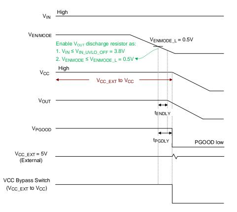
Figure 10. Power-Off Sequence of RT6310A/AH/D/DH: Ramping Down VEN/MODE
