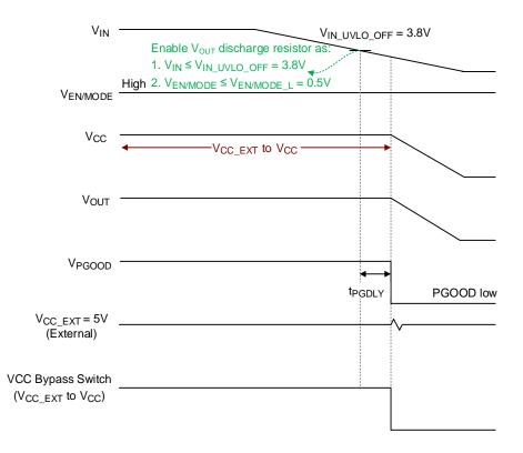
Figure 7. Power-Off Sequence of RT6310A/AH/D/DH: Ramping Down VIN
