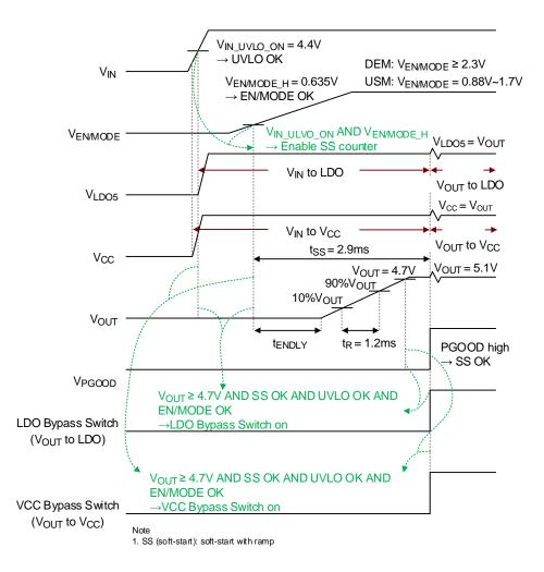
Figure 6. Power-On Sequence of RT6310C/CH: Ramping Up VIN Followed by VEN/MODE
