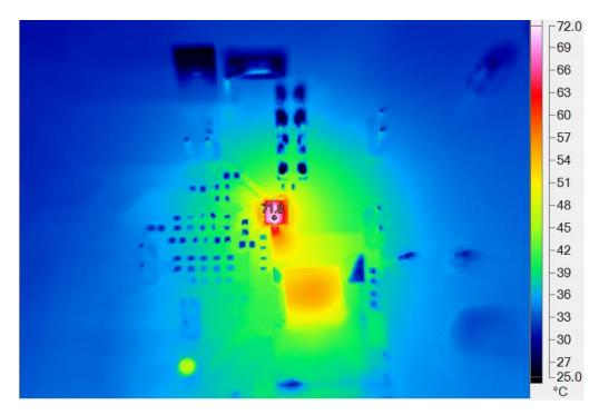
Figure 24. Thermal image of RT6310A/AH/D/DH with VOUT = 1.05V, VIN = 19V, IOUT = 10A and VCC\_EXT = 5V
