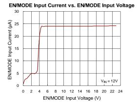
Figure 3. Characteristics of EN/MODE Input Current
