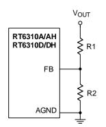
Figure 15. Output Voltage Setting
