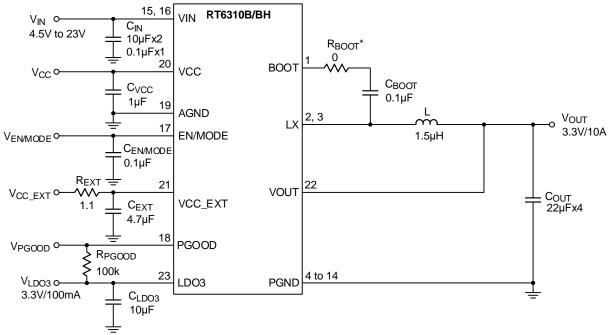
$R_{BOOT}^*$ :  $R_{BOOT}$  is reserved for option.  $R_{BOOT}$  must be less than 10 $\Omega$ .
