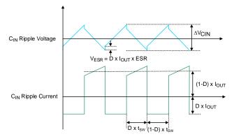
Figure 14. CIN Ripple Voltage and Ripple Current
