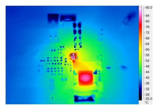
Figure 26. Thermal image of RT6310C/CH with Vout = 5.1V, VIN=19V, IOUT = 10A
