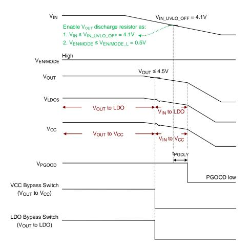
Figure 9. Power-Off Sequence of RT6310C/CH: Ramping Down VIN
