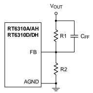
Figure 16. RT6310A/AH/D/DH Feedback Loop with Feedforward Capacitor
