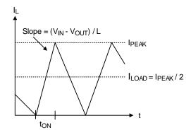
Figure 2. Boundary Condition of CCM/DEM
