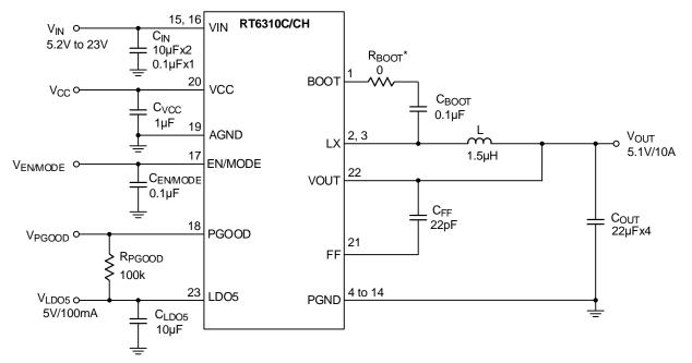
$R_{BOOT}^*$ :  $R_{BOOT}$  is reserved for option.  $R_{BOOT}$  must be less than 10 $\Omega$ .
