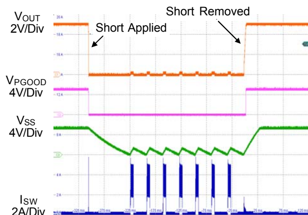
Figure 3. Short Circuit Protection and Recovery
