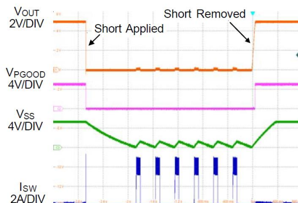
Figure 1. Short-Circuit Protection and Recovery
